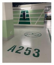
On level P1, some of the corridors provide one-way passage, while the dead-end layouts and the corridors leading to the ramp between levels require two-way traffic. In the dead-end layout, the possibility of turning around is provided.
